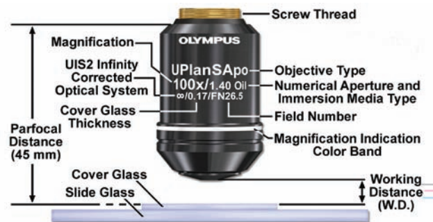
FIG. 84 Modern microscope objective specifications and nomenclature, including the definition for parfocal and working distances. A constant parfocal distance between similar objectives in a nose-piece ensures that each objective of increasing magnification will be in approximately the same focus as the others. Working distance is a measure of the free space between the objective front lens and the cover glass or specimen.
